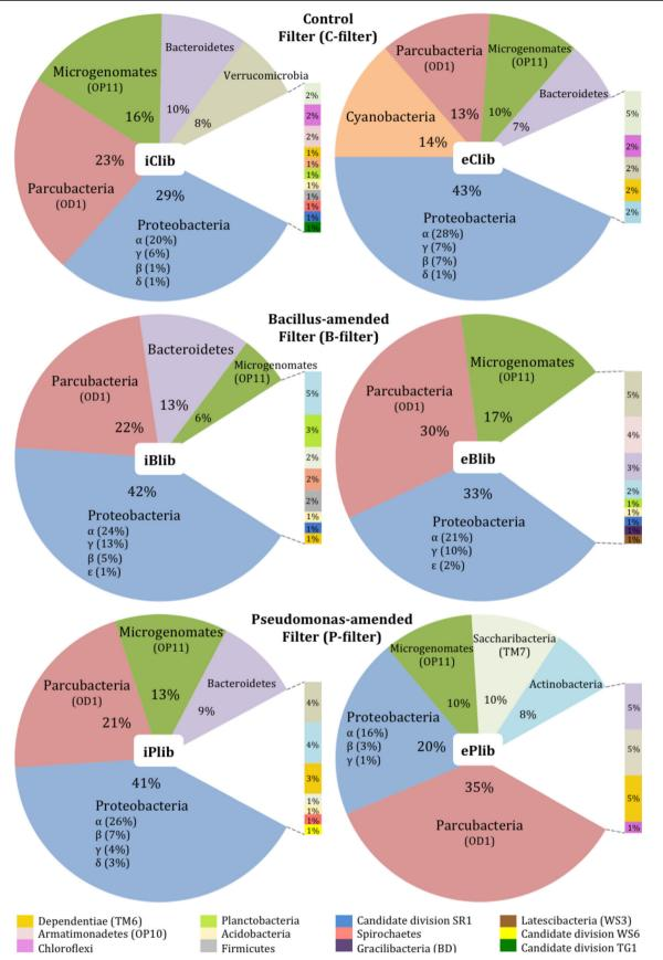
Fig. 4 Phylogenetic distributions of the six clone libraries constructed from nutrient solutions sampled in July in the influents and effluents of C-filter (iClib, eClib), B-filter (iBlib, eBlib), and P-filter (iPlib, ePlib)
